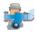
When the pump starts, the valve is open. The jet stream passing through the valve creates a negative pressure in the ball chamber relative to the pressure in an oil-filled chamber beneath the membrane.
