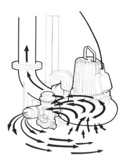
When the pump starts, the valve opens for approximately 30 seconds, shooting out a powerful jet stream that flushes all solids into suspension, ready to be pumped away.
