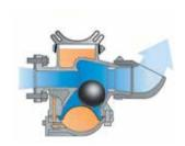
During the next 20 seconds, the ball is lifted by the membrane as the pressure in the two chambers equalizes. The time this takes can be varied by regulating the oil flow from the oil reservoir to the chamber beneath the membrane.
