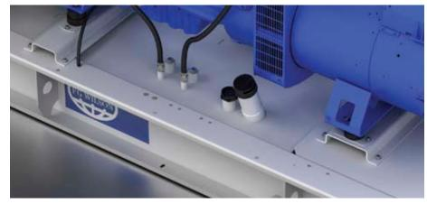
A wide fuel fill neck on the base frame allows easy access and fill by the operator, avoiding spills. The fuel tank is designed for 8 hours running at full load in prime applications. The top of the tank acts as a catchment area for all potential liquid spills and leaks.
