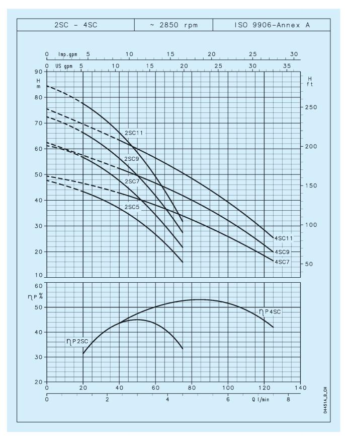
These performances are valid for liquids with density  $\rho=1.0 \text{ kg/dm}^3$  and kinematic viscosity  $\gamma=1 \text{ mm}^2/\text{sec}$ .
