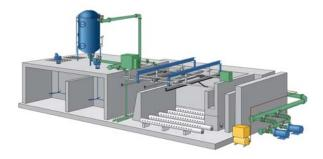
that works in tandem with the membrane filtration system. The DAF (dissolved air flotation) pretreatment overcomes problems often encountered in surface water sources and improves the efficiency of the 0.02-micron ZeeWeed 1000D membrane filter system provided by GE Water. The filtration membranes safeguard against pathogens that can pass through traditional sand/diatomaceous (S/D) filter systems.
