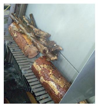
The screen rack is cleaned by very robust high-capacity rakes. The number of cleaning rakes can be variably adapted, removal capacity is then adjustable. Even extremely bulky objects are reliably removed by the screen rakes and transported upwards out of the channel to the screenings discharge.
