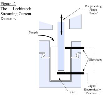
Suspended particles are adsorbed onto the walls under the action of Van der Waal's and electrostatic forces, see <u>Figure 3</u>. As the sample is moved rapidly back and forth, mobile counter ions, surrounding the charged particles, or colloids, are sheared near the surface of the particle and moved past the electrodes.
