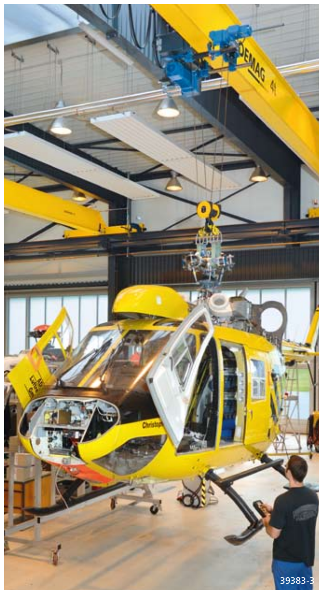
Demag rope hoists move helicopters into position for maintenance.
