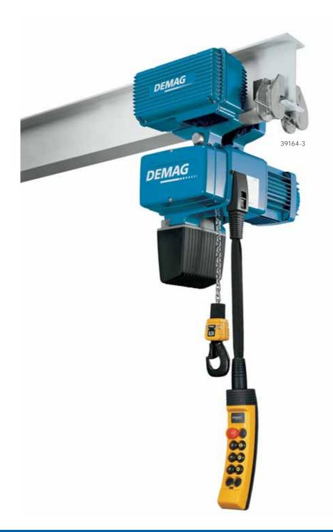
The drive is simply connected to the DC-Pro chain hoist using plug connectors and operated by means of the newly developed DSE 10-C control pendant. The control pendant for long and cross travel is simply fitted by means of a connector. The E 22 travel drive is used as standard for the KBK rail system with the new RF 125 friction wheel travel drive.
