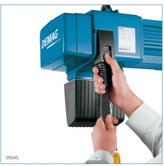
Height adjustment of the control cable
