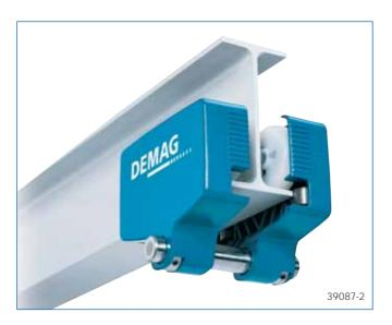
The lateral steel guide rollers support their curvenegotiating properties down to the minimum radius of 1000 mm and minimise girder wear. A drop-stop arrangement is integrated into the side cheeks, which consist of aluminium die-castings with a powder-coated finish.
