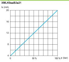
Connector wiring: 2-wire technique (4-20 mA)
