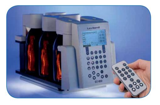
The unit is easy to use and set up using scrolling menus on the LCD display. Results can be monitored throughout the incubation period to ensure accurate analysis. With a selectable automatic start function, variations in sample temperature prior to testing can be eliminated, as the unit will begin the analysis period only when the temperature is constant. Such variations would normally cause errors during manometric measurement.
